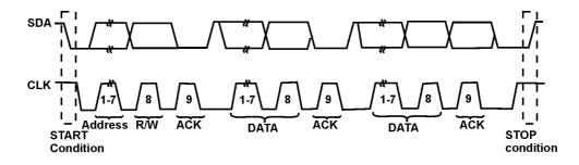
Depending on the status of the bit  $R/\overline{W}$ , two types of transmission are possible:
