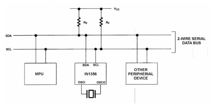
Data transfer can be start only when the bus is not busy. In the process of the data transfer the data line should remain stable, while the cycle signal line is in the high level status. Alterations of the data line status at that moment, when the cycle line is in the high status, will be understood as the control signals.
