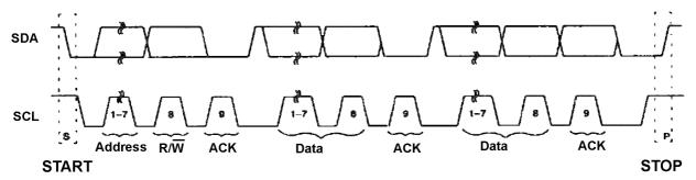
Depending on the status of bit  $R/\overline{W}$ , there are possible two types of transfer:
