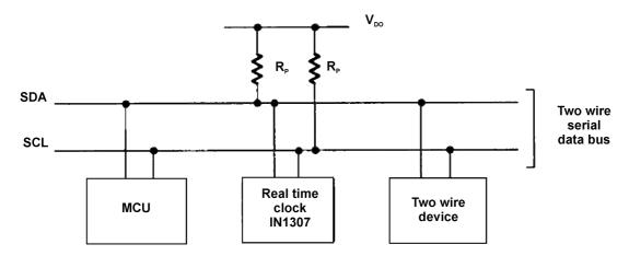
Data transfer can be initiated only when the bus is not occupied. In the process of the data transfer the data line should remain stable, while the line of the cycle signal is in the high status. Status alterations of the data line at that moment, when the cycle line is in the high status, will be regarded as the control signals.
